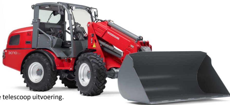
3070CX LP Telescoop, win/win situatie: lage machine, lange hefarm.
